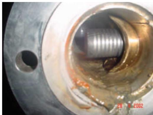
FIGURE 5 - View of Probe Installed in Tap
