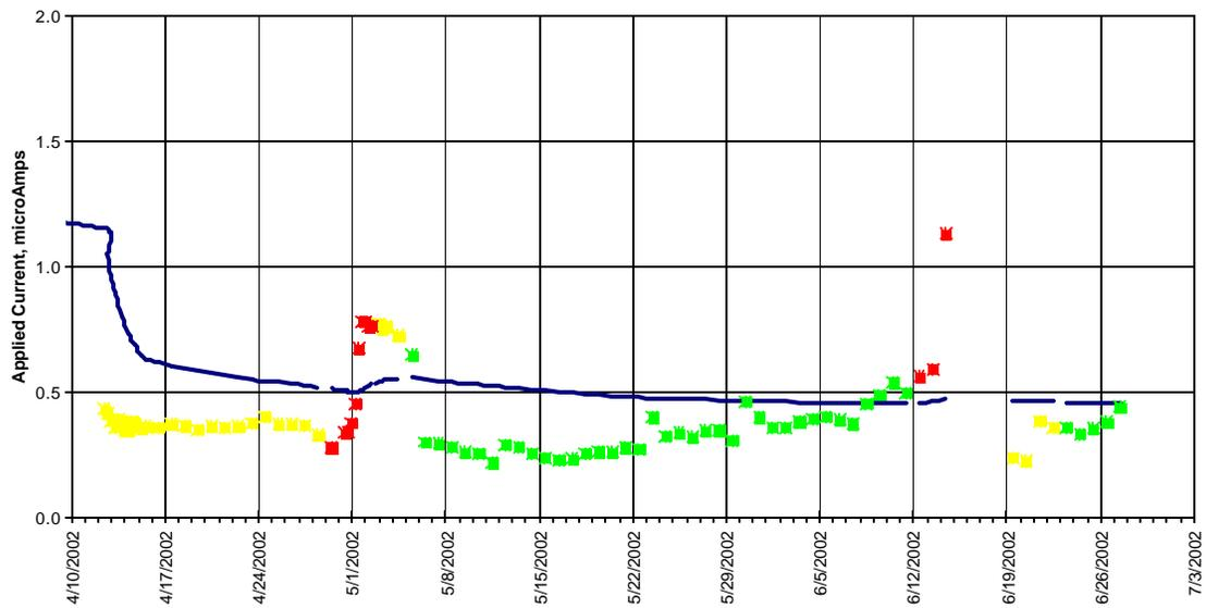
FIGURE 6 - Applied Current Trend – April 2002-June 2002 (Color code: Yellow = baseline being established; Green = probe is clean; Red = probe is fouled)
