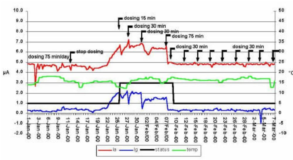
FIGURE 3 - Results from Biofilm Optimisation Study – Brackish Water-cooled Incineration Plant (from Reference 2)
